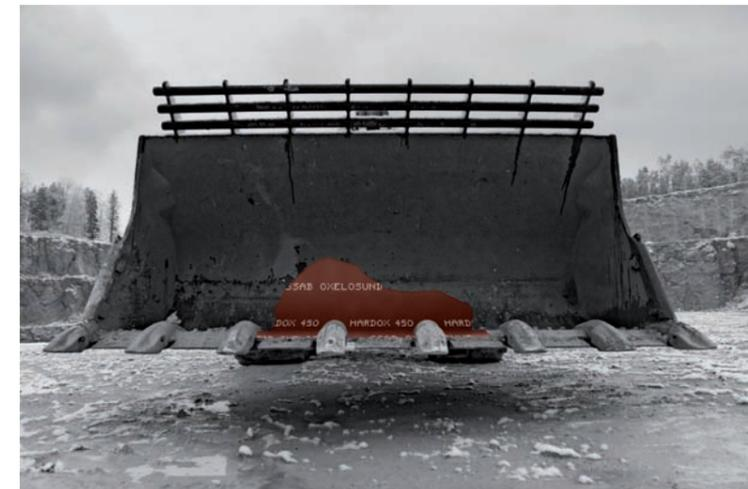
The various hardness grades of Hardox steel have optimum locations in the bucket. Hardox 450, for example, is very well suited for the body of the bucket, while Hardox 500 is appropriate for the cutting edge. Hardox HiTuf is eminently well suited for very thick cutting edges of large buckets.
